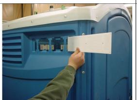
Install plastic expanding Rivets PN# 15337 into the 2 outside holes of each screen from the inside of the unit.
