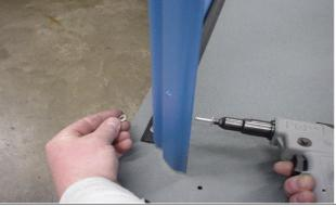
Rivet rear panel to left and right side panel using #68 large flange aluminum rivet install from outside of panel, through the 5th hole up from the bottom of both panels & back-up washer on the inside of panels.
