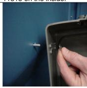
Insert the spindle PN# 16844 into the paperguard. Note the position of the hook.
