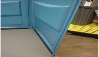
Finish installing remaining rivets & back-up washers in angles/panels. \*Tip: a standard flat blade screwdriver may be needed to pry bottom of panel up over exposed rivet/back-up washer attaching angle to floor.
