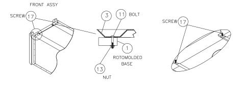
**DIRT BUSTER BASE:** INSTALL LAG SCREWS USING A 3/8 NUT DRIVER BIT AND DRILL. FASTEN SCREWS IN HOLES CLOSEST TO DOOR OPENING. MEASURE 2-1/4 FROM THAT SCREW AND FASTEN SECOND SCREWS IN NEW LOCATION. **SEE PICTURE.** REMOVE SHIPPING SCREW. OPEN DOOR AND INSTALL THE (2) LAG SCREWS TO DIMPLES TO INSIDE THE FACING FRAME. (TIGHTEN LAG SCREW UNTIL RUBBER WASHER BEGINS TO FLATTEN - DO NOT OVER TIGHEN).
