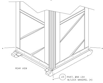
\*NOTE; IF UNIT IS ASSEMBLED WITH WOOD OR RECYCLED BASE, DRILL A 1/4" DIAMETER x 1/2" DEEP RELIEF HOLE INTO BASE USING THE LOWER HOLE IN THE PANEL AS A GUIDE.
