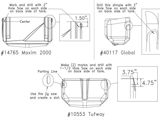
3. Insert hoses from Base Assy in drilled holes.
